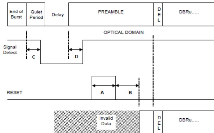
**Reset Signal Timing Diagram in Ranging Mode**
