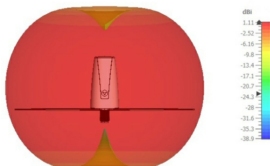
TYPICAL RADIATION PATTERN 1710 MHZ
