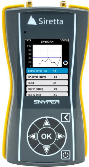
Surveying all network technologies, except for 5G NSA cells, does not need a SIM card. However, due to the specific way 5G NSA operates, a valid 5G SIM card is required. The SNYPER device will then display the 5G NSA cells of the network that the SIM card operates on.
