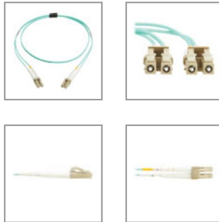
Rated OM4, this 50/125 multimode fiber cable with duplex LC connectors carries signals in 40/100 Gb Ethernet networks.
