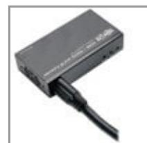
Transmit HDMI video and audio, RS-232 serial and IR Remote Control signals over a single Cat5e/6/6a cable to a projector, monitor or television. Ideal for digital signs and trade show presentations.
