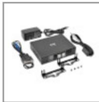
Receives IP-based audio + video signal transmitted point-to-point from a source 328 ft. away via Cat5e/6 cable or through a dedicated Ethernet network switch.
