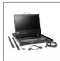
Control up to 16 computers with a single KVM switch with integrated console, or increase the total connected computers to 256 by daisy-chaining. This KVM switch is a smart solution for space- and money-saving server control.
