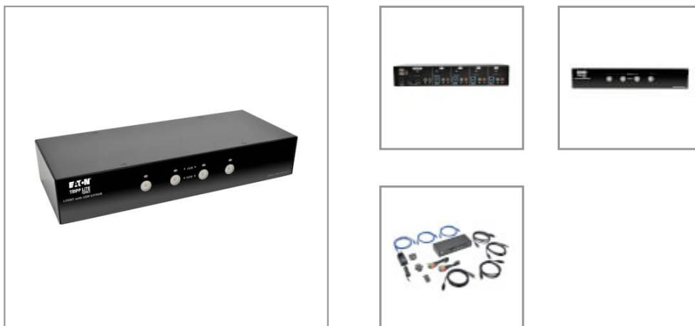
Control 4 DisplayPort computers using one DisplayPort monitor, USB keyboard and USB mouse. Connect USB 3.0 peripherals, such as hard drives and webcams, and share them between computers.
