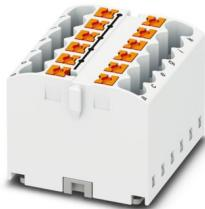
Distribution block, Basic terminal block, nom. voltage: 450 V, nominal current: 24 A, number of connections: 12, connection method: Push-in connection, cross section: 0.14 mm<sup>2</sup> - 4 mm<sup>2</sup>, mounting type: adhesive, color: white
