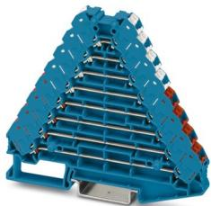
Potential distributors, without actuating push button, nom. voltage: 250 V, nominal current: 17.5 A, connection method: Push-in connection, 1st, 2nd, 3rd and 4th level, Rated cross section: 1.5 mm<sup>2</sup>, cross section: 0.14 mm<sup>2</sup> - 2.5 mm<sup>2</sup>, mounting: NS 35/7,5, NS 35/15, color: blue, color of connection elements: white, red
