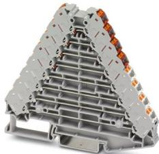
Marshalling panel, nom. voltage: 250 V, nominal current: 8 A, connection method: Push-in connection, 1st, 2nd, 3rd, 4th, 5th, 6th, 7th and 8th level, Rated cross section: 1.5 mm<sup>2</sup>, cross section: 0.14 mm<sup>2</sup> - 2.5 mm<sup>2</sup>, mounting: NS 35/7,5, NS 35/15, color: gray, color of connection elements: red, white
