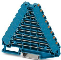
Marshalling panel, nom. voltage: 250 V, nominal current: 8 A, connection method: Push-in connection, 1st, 2nd, 3rd, 4th, 5th, 6th, 7th and 8th level, Rated cross section: 1.5 mm<sup>2</sup>, cross section: 0.14 mm<sup>2</sup> - 2.5 mm<sup>2</sup>, mounting: NS 35/7,5, NS 35/15, color: blue, color of connection elements: blue
