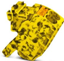
Pick-off terminal block, nom. voltage: 1500 V, nominal current: 57 A, number of connections: 2, connection method: Push-in connection, Rated cross section: 10 mm<sup>2</sup>, 1 level, cross section: 0.5 mm<sup>2</sup> - 16 mm<sup>2</sup>, mounting type: on base element, color: black/yellow
