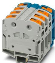
High-current terminal block, Blocked, nom. voltage: 1000 V, nominal current: 232 A, number of connections: 8, number of positions: 4, connection method: PowerTurn connection, cross section: 25 mm<sup>2</sup> - 95 mm<sup>2</sup>, mounting type: NS 35/15, color: gray/blue
