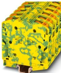
Protective conductor terminal block, number of connections: 2, number of positions: 1, connection method: PowerTurn connection, Rated cross section: 95 mm<sup>2</sup>, cross section: 25 mm<sup>2</sup> - 95 mm<sup>2</sup>, mounting type: 2.3 mm copper DIN rail, color: green-yellow
