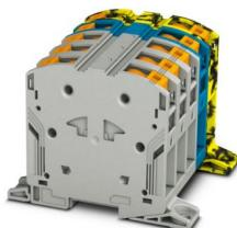
High-current terminal block, Blocked, nom. voltage: 1000 V, nominal current: 150 A, number of connections: 10, number of positions: 5, connection method: PowerTurn connection, 1 level, cross section: 10 mm<sup>2</sup> - 70 mm<sup>2</sup>, mounting type: direct screw connection, color: gray/blue/black-yellow
