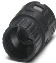
Corrugated pipe adapter, with internal thread, for connecting corrugated pipes to HEAVYCON EVO M40 plastic cable glands or ADVANCE M40 plastic housings, straight, black, IP66.
