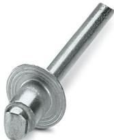
Blind rivets, Ø 4.8 mm, 6 mm sleeve length, aluminum sleeve, zinc-plated steel pin, flat head, standard version similar to DIN 7337 A
