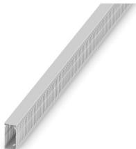
Cable duct for installation and mounting in control cabinets, gray, comprising upper part and mounting base, width: 30 mm, height: 60 mm, length: 2000 mm
