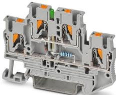
Double-level terminal block, nom. voltage: 500 V, nominal current: 0.1 A, 1st and 2nd level, connection method: Push-in connection, Rated cross section: 2.5 mm<sup>2</sup>, cross section: 0.14 mm<sup>2</sup> - 4 mm<sup>2</sup>, mounting: NS 35/7,5, NS 35/15, color: gray
