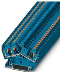
Feed-through terminal block, nom. voltage: 800 V, nominal current: 32 A, number of connections: 3, connection method: Push-in connection, Rated cross section: 4 mm<sup>2</sup>, 1 level, cross section: 0.2 mm<sup>2</sup> - 6 mm<sup>2</sup>, mounting type: NS 35/7,5, NS 35/15, color: blue
