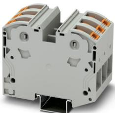
High-current terminal block, Blocked, nom. voltage: 1000 V, nominal current: 125 A, number of connections: 6, number of positions: 3, connection method: PowerTurn connection, Rated cross section: 35 mm<sup>2</sup>, cross section: 2.5 mm<sup>2</sup> - 35 mm<sup>2</sup>, mounting type: NS 35/15, color: gray
