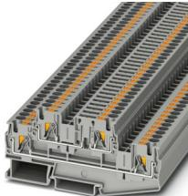
Disconnect terminal block, Current and voltage are determined by the plug used., nom. voltage: 500 V, nominal current: 28 A, 1 level, connection method: Push-in connection, Rated cross section: 4 mm<sup>2</sup>, cross section: 0.2 mm<sup>2</sup> - 6 mm<sup>2</sup>, 2nd level, connection method: Push-in connection, Rated cross section: 4 mm<sup>2</sup>, cross section: 0.2 mm<sup>2</sup> - 6 mm<sup>2</sup>, mounting: NS 35/7,5, NS 35/15, color: gray
