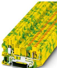
Protective conductor terminal block, connection method: Push-in connection, cross section: 0.2 mm<sup>2</sup> - 6 mm<sup>2</sup>, connection method: Screw connection, cross section: 0.14 mm<sup>2</sup> - 6 mm<sup>2</sup>, mounting: NS 35/7,5, NS 35/15, color: green-yellow
