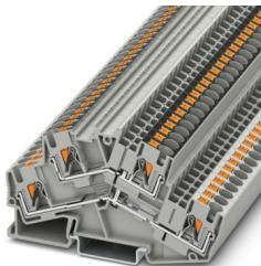
Double-level terminal block, with equipotential bonder, nom. voltage: 800 V, nominal current: 28 A, connection method: Push-in connection, 1st and 2nd level, Rated cross section: 4 mm<sup>2</sup>, cross section: 0.2 mm<sup>2</sup> - 6 mm<sup>2</sup>, mounting type: NS 35/7,5, NS 35/15, color: gray
