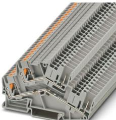
Double-level terminal block, nom. voltage: 800 V, nominal current: 22 A, number of connections: 4, connection method: Push-in / plug connection, Rated cross section: 2.5 mm<sup>2</sup>, 1st and 2nd level, cross section: 0.14 mm<sup>2</sup> - 4 mm<sup>2</sup>, mounting type: NS 35/7,5, NS 35/15, color: gray
