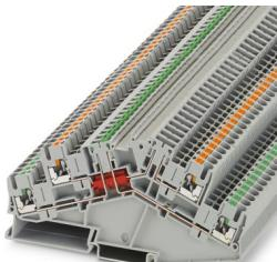
Disconnect terminal block, Current and voltage are determined by the plug used., Double level with angled contour, one disconnect knife, and one disconnect point, nom. voltage: 400 V, nominal current: 16 A, 1st and 2nd level, connection method: Push-in connection, Rated cross section: 2.5 mm<sup>2</sup>, cross section: 0.14 mm<sup>2</sup> - 4 mm<sup>2</sup>, mounting: NS 35/7,5, NS 35/15, color: gray
