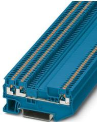
Feed-through terminal block, same shape as disconnect terminal block, nom. voltage: 400 V, nominal current: 17.5 A, number of connections: 3, connection method: Push-in connection, Rated cross section: 1.5 mm<sup>2</sup>, 1 level, cross section: 0.14 mm<sup>2</sup> - 1.5 mm<sup>2</sup>, mounting type: NS 35/7,5, NS 35/15, color: blue
