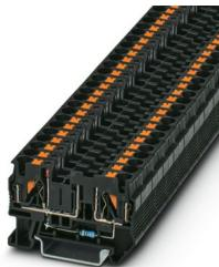
Fuse modular terminal block, fuse type: Blade, fuse type: ISO 8820-3 Type F (miniature), nom. voltage: 12 V DC, nominal current: 10 A, connection method: Push-in connection, Rated cross section: 4 mm<sup>2</sup>, cross section: 0.2 mm<sup>2</sup>- 6 mm<sup>2</sup>, mounting type: NS 35/7,5, NS 35/15, color: black
