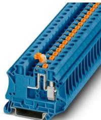
Knife-disconnect terminal block, With test socket screws for insertion of test plugs, nom. voltage: 500 V, Thermal continuous current  $I_{th}$ : 20 A, connection method: Screw connection, Rated cross section: 6 mm<sup>2</sup>, cross section: 0.2 mm<sup>2</sup> - 10 mm<sup>2</sup>, mounting: NS 35/7,5, NS 35/15, color: blue
