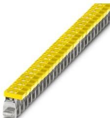
Connection terminal block, nom. voltage: 300 V, nominal current: 76 A, connection method: Screw connection, Rated cross section: 16 mm<sup>2</sup>, cross section: 1.5 mm<sup>2</sup> - 16 mm<sup>2</sup>, mounting: Neutral busbar, color: yellow
