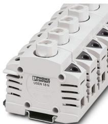
Fuse modular terminal block, fuse type: Screw cartridge, fuse type: D 02 / E 18, nom. voltage: 400 V, nominal current: 63 A, connection method: Screw connection, Rated cross section: 35 mm<sup>2</sup>, cross section: 1.5 mm<sup>2</sup> - 35 mm<sup>2</sup>, mounting type: NS 35/7,5, NS 35/15, color: light gray
