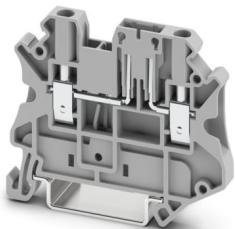
Disconnect terminal block, Current and voltage are determined by the plug used., With test socket screws for insertion of test plugs, nom. voltage: 400 V, nominal current: 20 A, Thermal continuous current  $I_{th}$ : 20 A, connection method: Screw connection, Rated cross section: 2.5 mm<sup>2</sup>, cross section: 0.14 mm<sup>2</sup> - 4 mm<sup>2</sup>, mounting: NS 35/7,5, NS 35/15, color: gray
