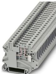
Disconnect terminal block, Current and voltage are determined by the plug used., With test socket screws for insertion of test plugs, nom. voltage: 500 V, nominal current: 20 A, connection method: Screw connection, Rated cross section: 4 mm<sup>2</sup>, cross section: 0.14 mm<sup>2</sup> - 6 mm<sup>2</sup>, mounting: NS 35/7,5, NS 35/15, color: gray
