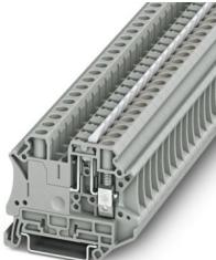
Knife-disconnect terminal block, with actuation latch, white disconnect knife, and test socket screws for insertion of test plugs, nom. voltage: 500 V, nominal current: 20 A, connection method: Screw connection, Rated cross section: 2.5 mm<sup>2</sup>, cross section: 0.2 mm<sup>2</sup> - 10 mm<sup>2</sup>, mounting: NS 35/7,5, NS 35/15, color: gray
