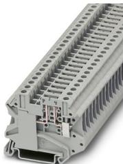
Disconnect terminal block, Current and voltage are determined by the plug used., nom. voltage: 500 V, nominal current: 20 A, connection method: Screw connection, Rated cross section: 4 mm<sup>2</sup>, cross section: 0.14 mm<sup>2</sup> - 6 mm<sup>2</sup>, mounting: NS 35/7,5, NS 35/15, color: gray
