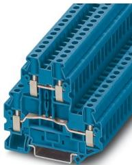
Double-level terminal block with a screw connection, cross section: 0.14 mm<sup>2</sup> - 6 mm<sup>2</sup>, AWG: 26 - 10, width: 6.2 mm, color: blue
