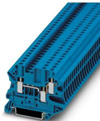
Feed-through terminal block, nom. voltage: 500 V, nominal current: 24 A, number of connections: 3, connection method: Screw connection, Rated cross section: 2.5 mm<sup>2</sup>, 1 level, cross section: 0.14 mm<sup>2</sup> - 4 mm<sup>2</sup>, mounting type: NS 35/7,5, NS 35/15, color: blue
