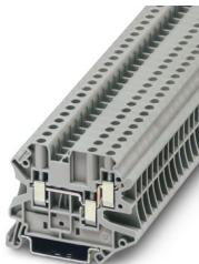
Feed-through terminal block, nom. voltage: 500 V, nominal current: 32 A, number of connections: 3, connection method: Screw connection, Rated cross section: 4 mm<sup>2</sup>, cross section: 0.14 mm<sup>2</sup> - 6 mm<sup>2</sup>, mounting type: NS 35/7,5, NS 35/15, color: gray
