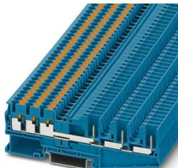
Feed-through terminal block, nom. voltage: 500 V, nominal current: 24 A, number of connections: 6, connection method: Push-in / plug connection, Rated cross section: 2.5 mm<sup>2</sup>, 1st, 2nd and 3rd level, cross section: 0.14 mm<sup>2</sup> - 4 mm<sup>2</sup>, mounting type: NS 35/7,5, NS 35/15, color: blue
