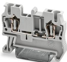
Feed-through terminal block, for installing components that can be individually selected, nom. voltage: 800 V, nominal current: 24 A, number of connections: 2, connection method: Spring-cage connection, Rated cross section: 2.5 mm<sup>2</sup>, 1 level, cross section: 0.08 mm<sup>2</sup> - 4 mm<sup>2</sup>, mounting type: NS 35/7,5, NS 35/15, color: gray
