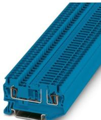
Disconnect terminal block, Current and voltage are determined by the plug used., nom. voltage: 400 V, nominal current: 20 A, connection method: Spring-cage connection, Rated cross section: 2.5 mm<sup>2</sup>, cross section: 0.08 mm<sup>2</sup> - 4 mm<sup>2</sup>, mounting: NS 35/7,5, NS 35/15, color: blue
