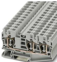
Feed-through terminal block, nom. voltage: 1000 V, nominal current: 57 A, number of connections: 3, connection method: Spring-cage connection, Rated cross section: 10 mm<sup>2</sup>, 1 level, cross section: 0.2 mm<sup>2</sup> - 16 mm<sup>2</sup>, mounting type: NS 35/7,5, NS 35/15, color: gray
