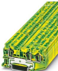
Protective conductor terminal block, number of connections: 3, number of positions: 1, connection method: Spring-cage connection, Rated cross section: 4 mm<sup>2</sup>, cross section: 0.08 mm<sup>2</sup> - 6 mm<sup>2</sup>, mounting type: NS 35/7,5, NS 35/15, color: green-yellow
