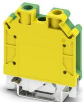
Protective conductor terminal block, number of connections: 2, connection method: Screw connection, Rated cross section: 10 mm<sup>2</sup>, cross section: 0.5 mm<sup>2</sup> - 16 mm<sup>2</sup>, mounting method: PE foot with mounting screw, M4, mounting type: NS 35/7,5, NS 35/15, NS 32, color: green-yellow
