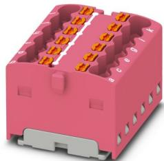
Distribution block, bridged internally, nom. voltage: 450 V, nominal current: 17.5 A, number of connections: 12, connection method: Push-in connection, cross section: 0.14 mm<sup>2</sup> - 2.5 mm<sup>2</sup>, mounting type: for snapping onto a DIN rail adapter, Direct mounting with flange, Free-hanging, color: pink
