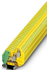
Protective conductor terminal block, When aligning with a feed-through terminal block of the same shape, an end cover must be interposed for insulation voltages of > 320 V, number of connections: 3, connection method: Screw connection, 1 level, cross section: 0.14 mm<sup>2</sup> - 1.5 mm<sup>2</sup>, mounting type: NS 15, color: green-yellow
