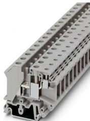
Feed-through terminal block, nom. voltage: 800 V, nominal current: 57 A, connection method: Screw connection, 1 level, Rated cross section: 10 mm<sup>2</sup>, cross section: 0.5 mm<sup>2</sup> - 16 mm<sup>2</sup>, Screw connection, 1st level connection right, Rated cross section: 4 mm<sup>2</sup>, cross section: 0.2 mm<sup>2</sup> - 6 mm<sup>2</sup>, mounting type: NS 35/7,5, NS 35/15, NS 32, color: gray
