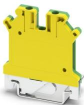
Protective conductor terminal block, number of connections: 2, number of positions: 1, connection method: Screw connection, cross section: 0.2 mm<sup>2</sup> - 4 mm<sup>2</sup>, mounting method: PE foot with mounting screw, M2.5, mounting type: NS 35/7,5, NS 35/15, NS 32, color: green-yellow
