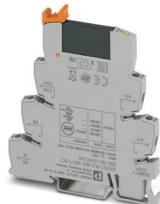
PLC-INTERFACE for output functions, consisting of PLC-BSC.../ACT basic terminal block with screw connection and plug-in miniature solid-state relay, for mounting on DIN rail NS 35/7,5, 1 N/O contact, input: 5 V DC, output: 3 - 33 V DC/3 A
